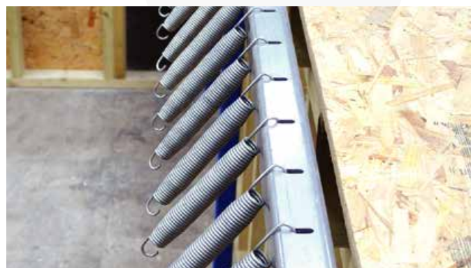
8.5" tapered springs with elongated hook in custom steel frame
